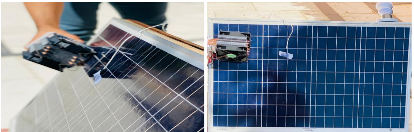
Figure 5. How to install thermoelectric heat sink on the solar panel (Source: Field study)
