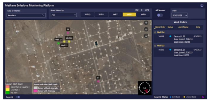
Figure 5. AI-enabled MEMP with real-time leak detection and WO management (Adapted from Microsoft, 2023)
